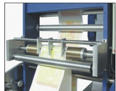
Details of "Cutting Unit" (multi-line)
